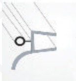
APS-5 Water Dispersal seal 8mm (2.2mtr.) 10mm (2.2mtr.) 12mm (2.2mtr.)
